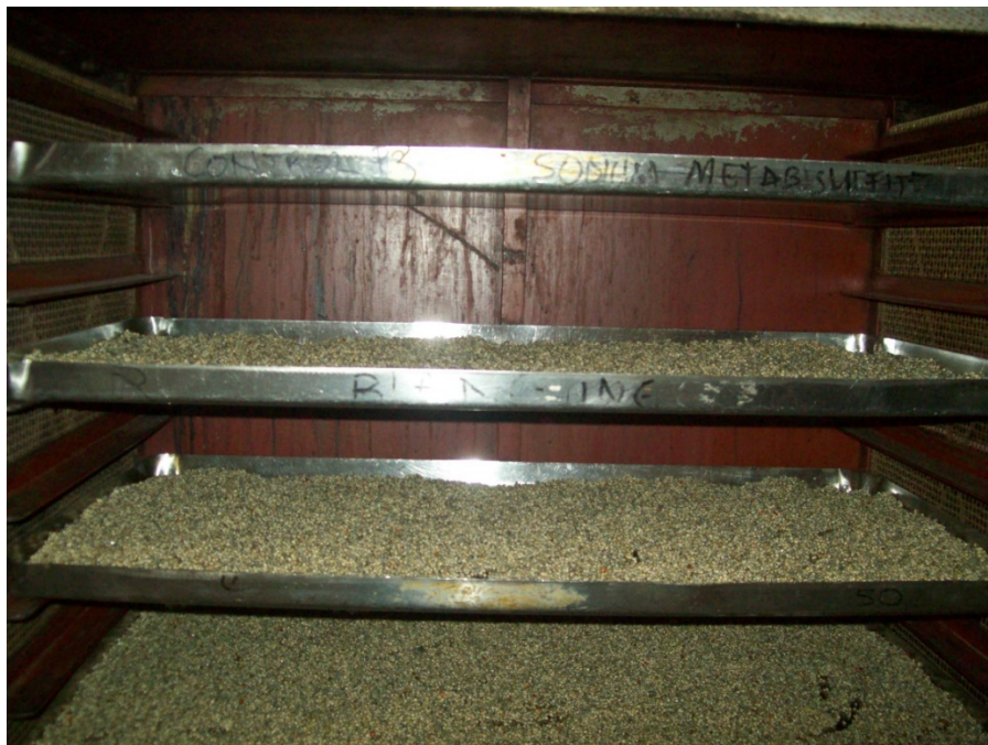
Drying of soaked grains in a mechanical dryer at 55°C
