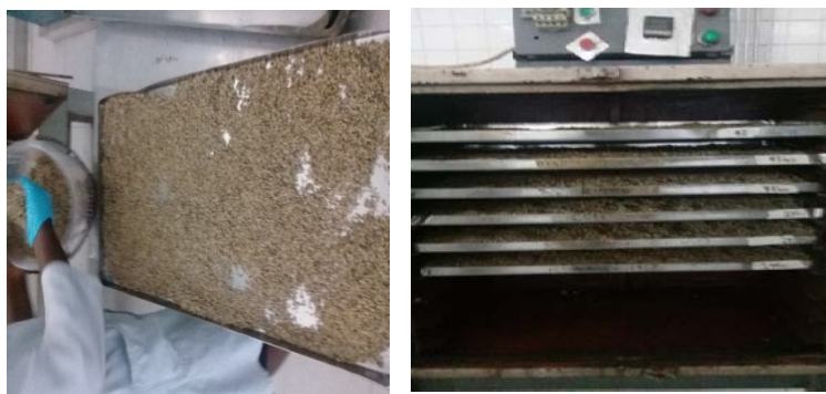
Figure 36: Drying of millet after soaking
