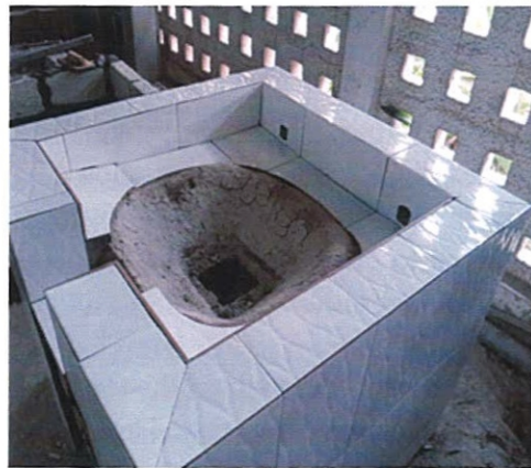
Figure 3B: Modified Ahotor oven with fat collector at CSIR-FRI
