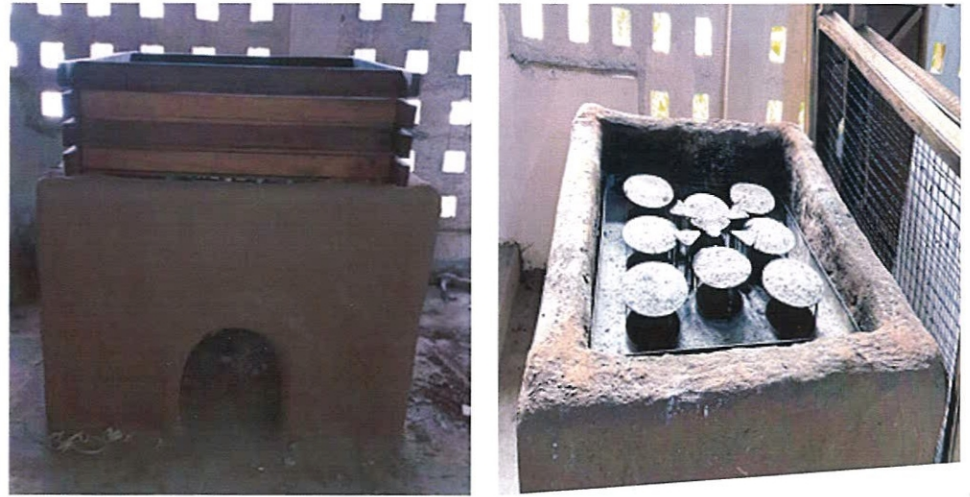
Figure 4: Modified chorkor oven with fat collector at CSIR-FRI
