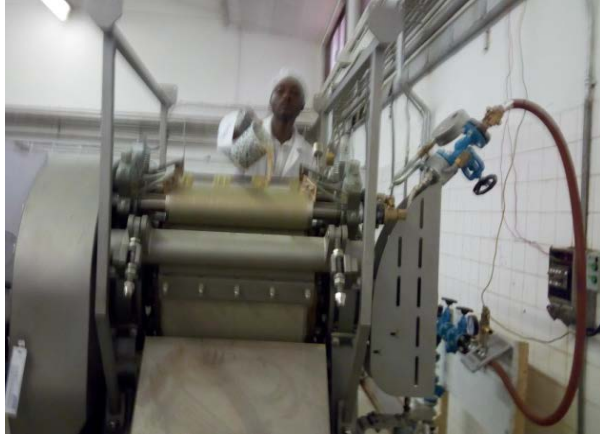
Picture 6: Feeding slurry into drum dry dryer
