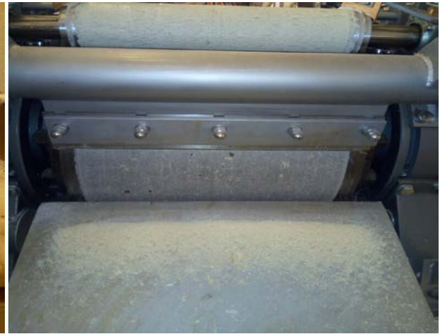
Picture 9: Blade scraping off dried product from the roller
