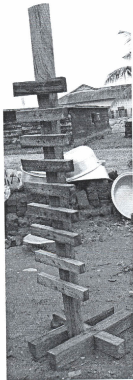
Fig. 21 Wooden support for metal trays
