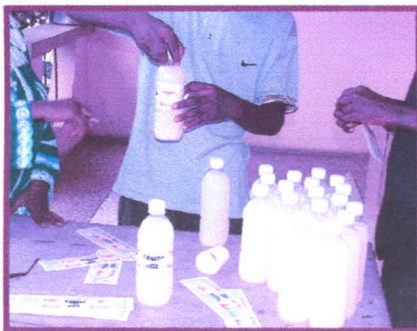
Fig. 3.56: This is the labeling step in the banana fruit juice production. The fruit juice bottled in clean bottles are labeled with a stickers showing product name, basic ingredients, dates of production and time period within which the product is good for consumption.
