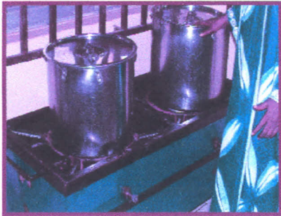
Fig. 3.55 Pasteurization step. It is done in stainless steel pans on gas stove. It is a batch process. It will be time consuming and there is the possibility of recontamination.
