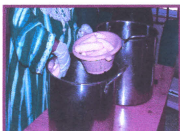
Fig. 3.50 Peeled fruits being taken out of the sodium metabisulphite solution. They are allowed to stay in a mesh so that the water get drained
