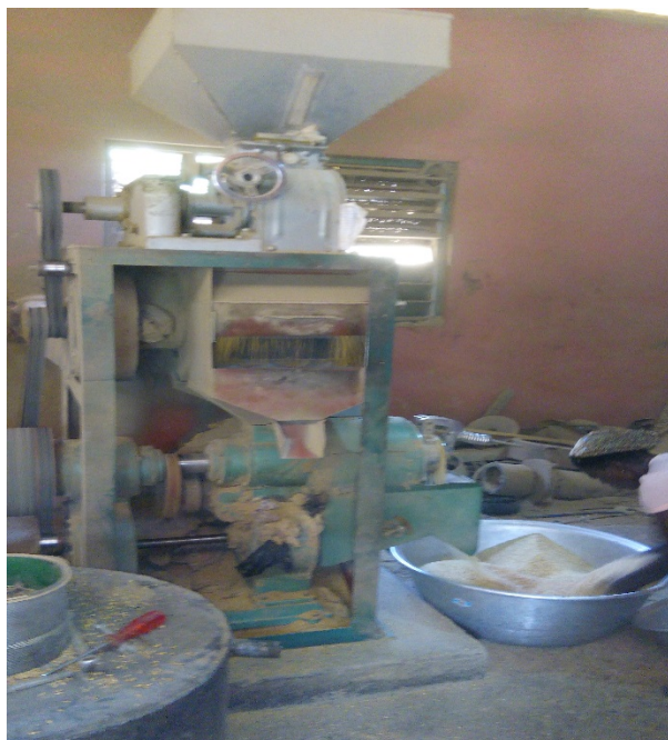
Milling of paddy using a roller mill
