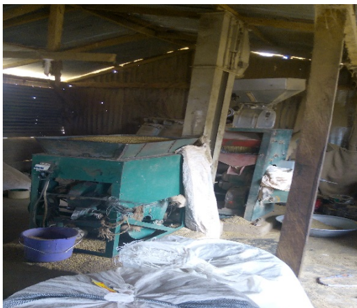
Milling of paddy using a roller mill
