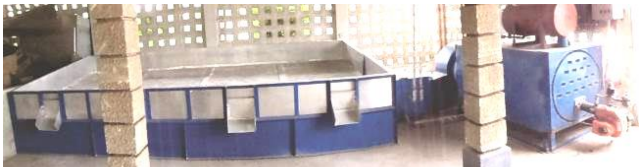
Figure 2. Bin dryer showing product outlet points
