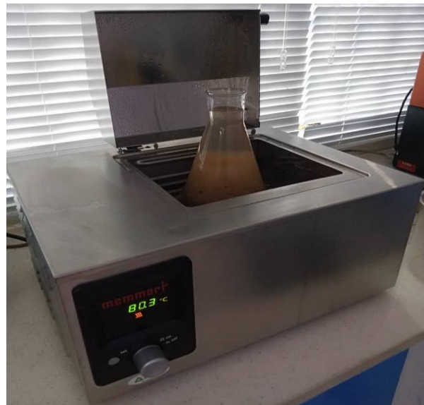
Extraction of gelatin in water bath
