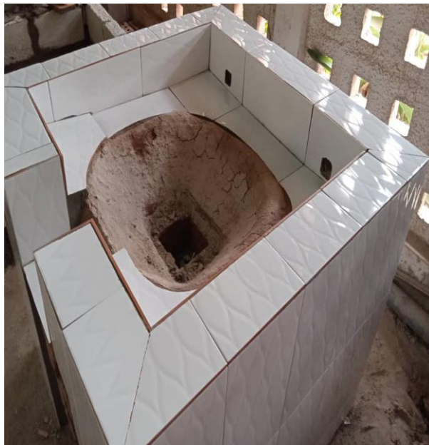
Gas, charcoal and fuelwood combined Ahotor oven
