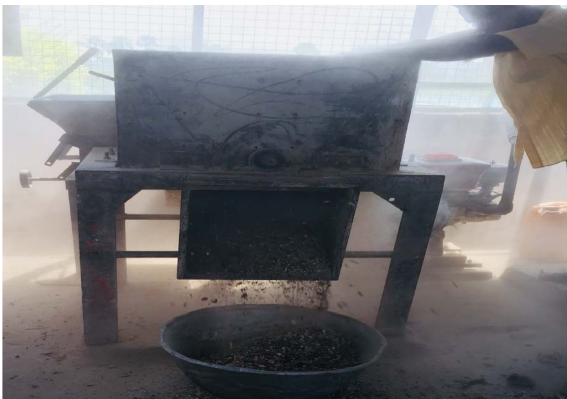
Figure 3: Milling of dried cassava peels
