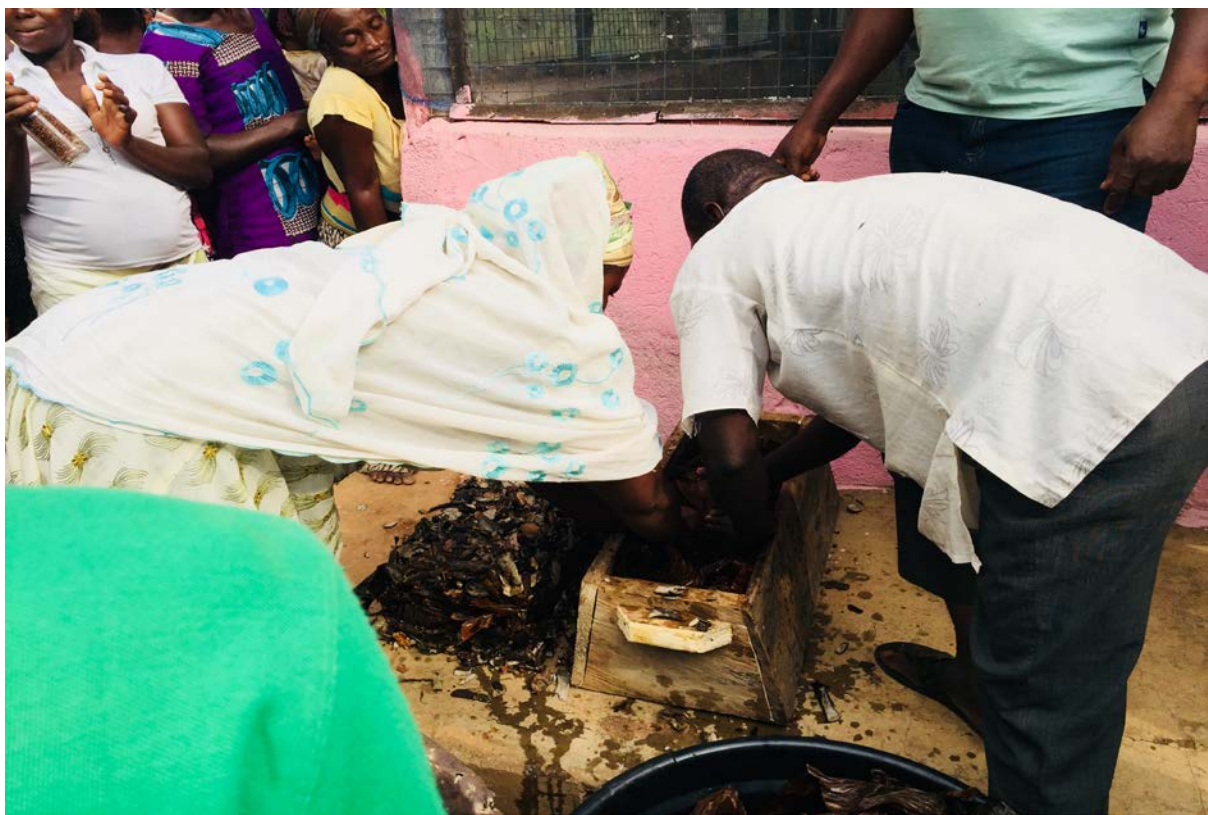
Figure 4: Stacking of cassava waste into mold.
