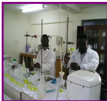
Fig. 2.4 Partitioning using the separating funnel
