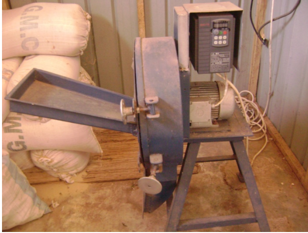
Figure 4: Grass cutting machine fabricated during the project
