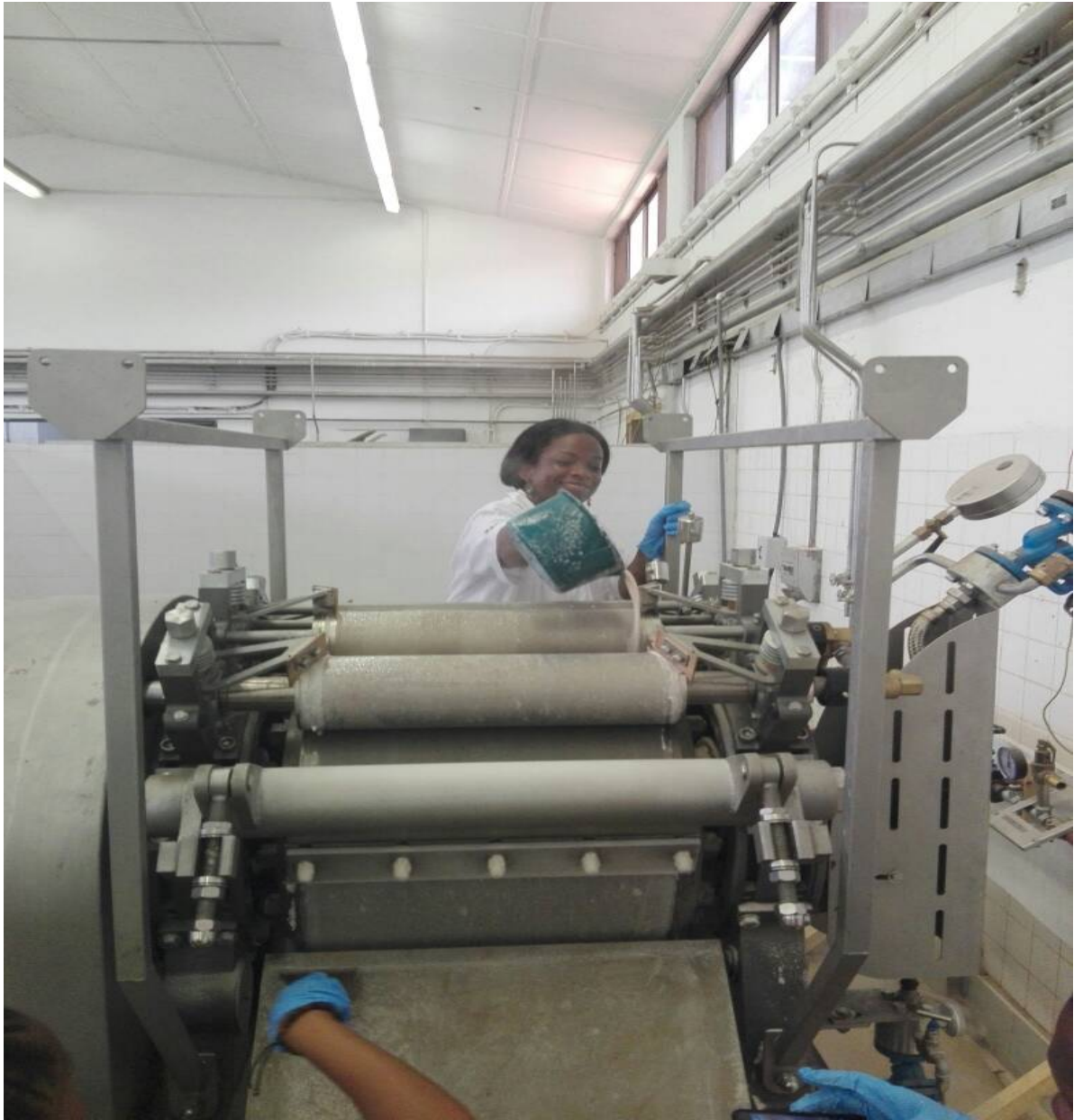
Figure 1: Drying of cocoyam slurry using the Andritz Gouda Contact drum dryer
