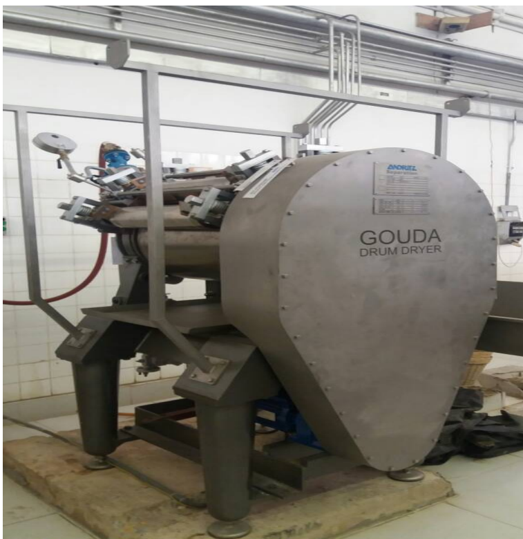
Figure 3: Andritz Gouda Contact drum dryer
